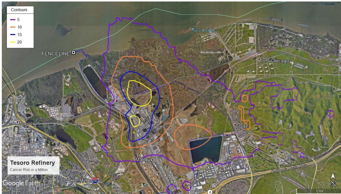
Figure E-16 - Estimated Cancer Risk from a 2015 Health Risk Assessment of Emissions from the Marathon Refinery
