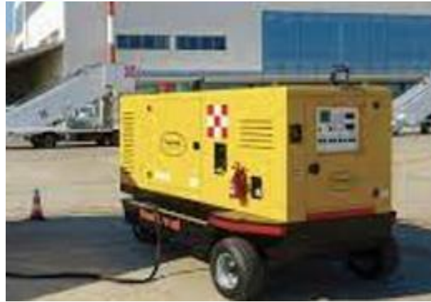
ground power unit
