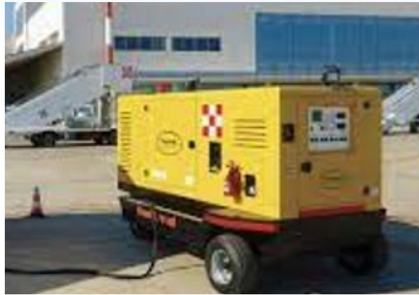
ground power unit
