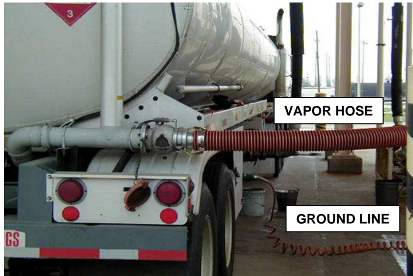
Figure 2 Tank Truck Connects to Vapor Hose
