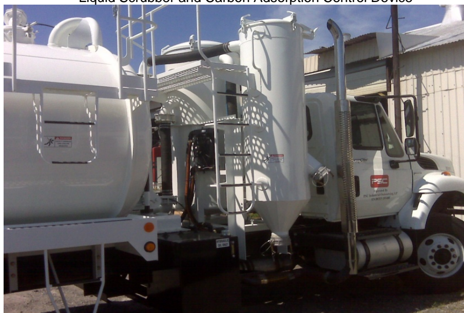
Figure 11 Vacuum Truck Containing a Combination of a Liquid Scrubber and Carbon Adsorption Control Device
