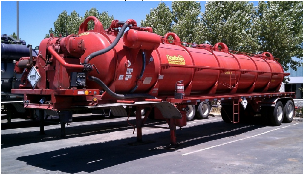
Figure 4 Vacuum Truck Trailer with a Fill Capacity of 9,000 Gallons
