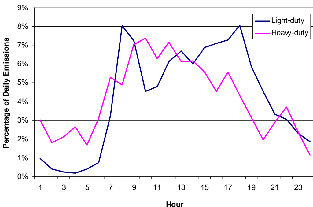
Figure 22. Diurnal profiles applied to emissions from light-duty and heavy-duty vehicles.
