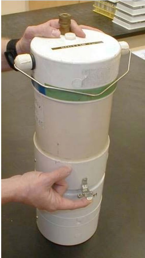
AirMetric MiniVolumetric Aerosol Sampler (20" long by 7" in diameter)
