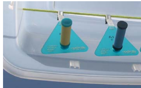
Radiello passive samplers for VOC, and aldehydes (size of a roll of pennies)
