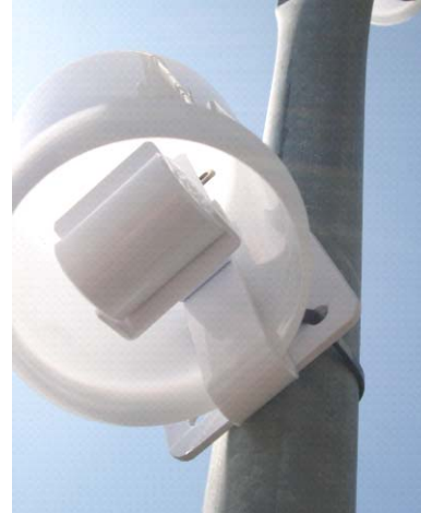
Ogawa passive samplers for NO x and SO 2 (thumb size in protective cup shield)
