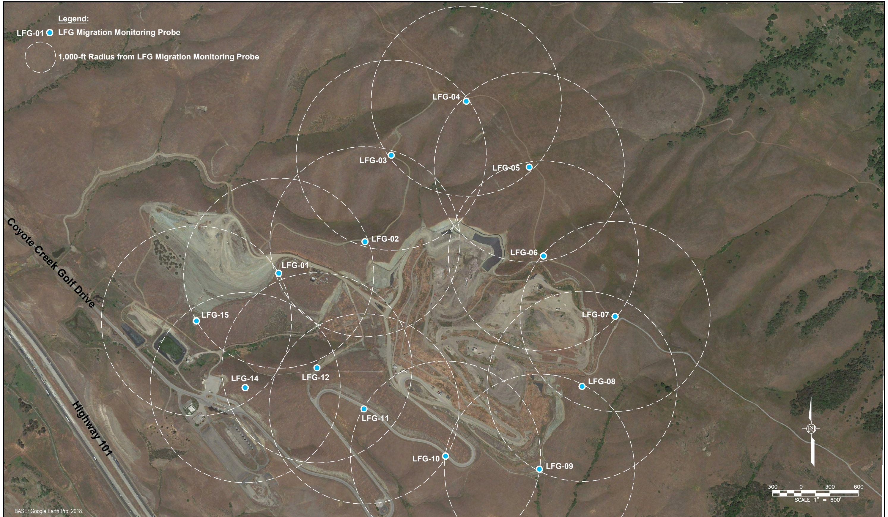
FIGURE 1 PERIMETER GAS PROBE LOCATIONS KIRBY CANYON RECYCLING & DISPOSAL FACILITY SANTA CLARA COUNTY, CALIFORNIA
