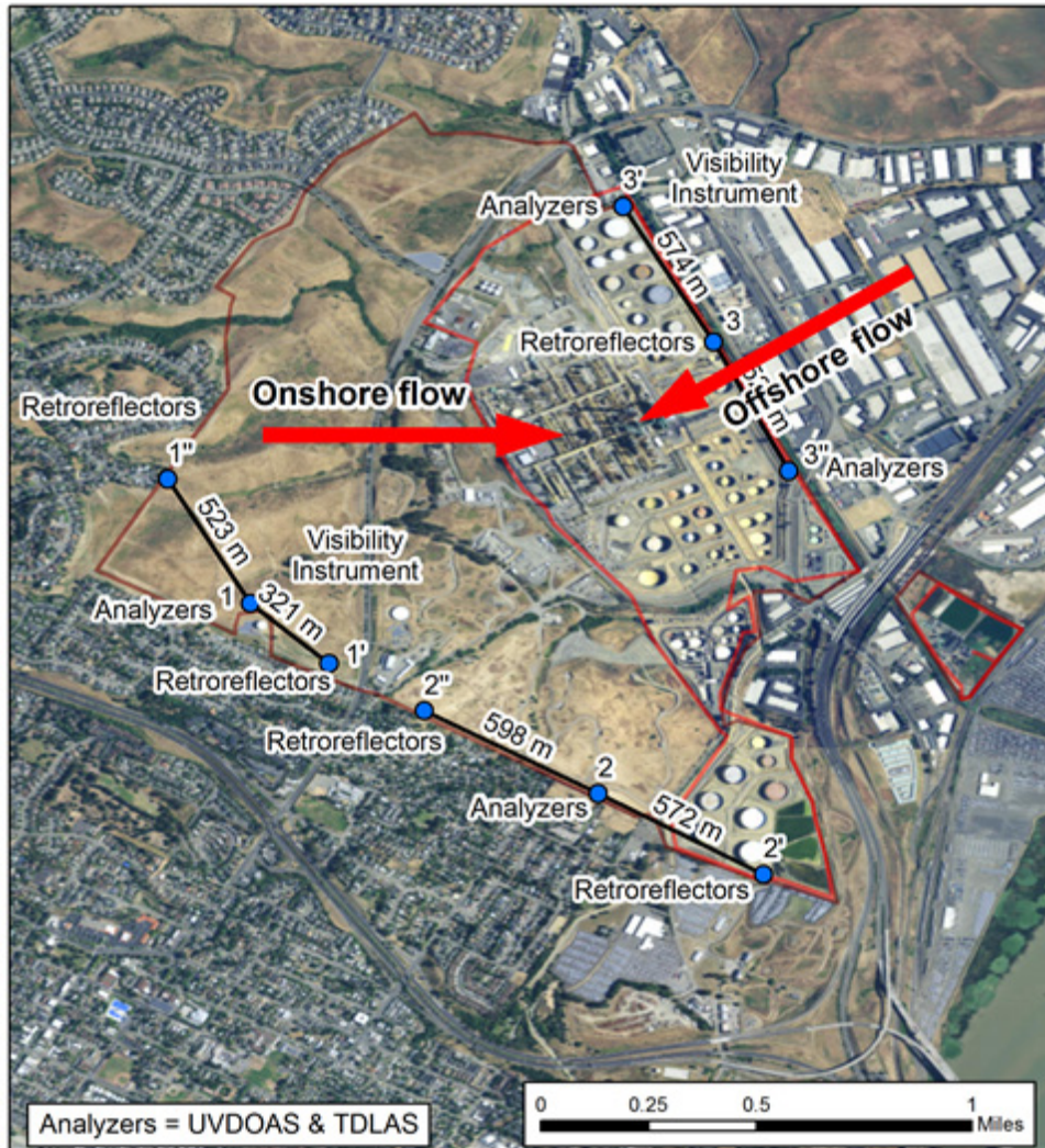
Figure 2. Open-path monitoring network for Valero's Benicia Refinery. Each primary path is numbered, and the sites are numbered and labeled with a prime (') or double prime (") symbol. Main wind flow directions are shown.
