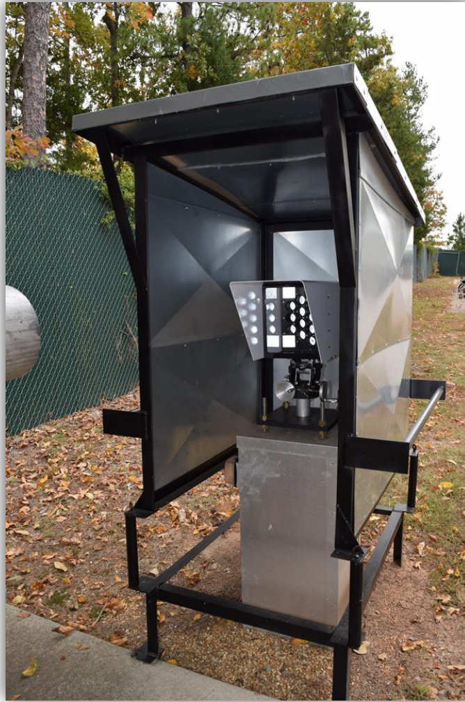
Figure 18. Example of a UV-DOAS retroreflector installation.
