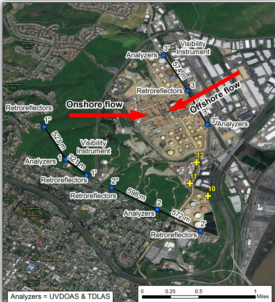
Figure 2. Proposed open-path monitoring network for Valero's Benicia Refinery. Each primary path is numbered and contains segments that are labeled with the path number and a prime (') or double prime (") symbol. Yellow "+" symbols indicate the location of point monitoring by sorbent tubes. Main wind flow directions are also shown.
