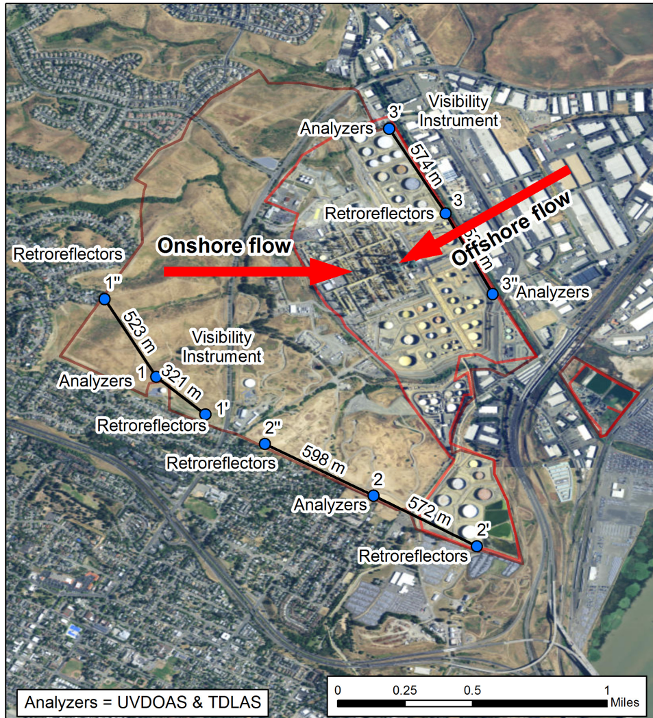
Figure 2. Proposed open-path monitoring network for Valero's Benicia Refinery. Each primary path is numbered and contains segments that are labeled with the path number and a prime (') or double prime (") symbol. Main wind flow directions are also shown.
