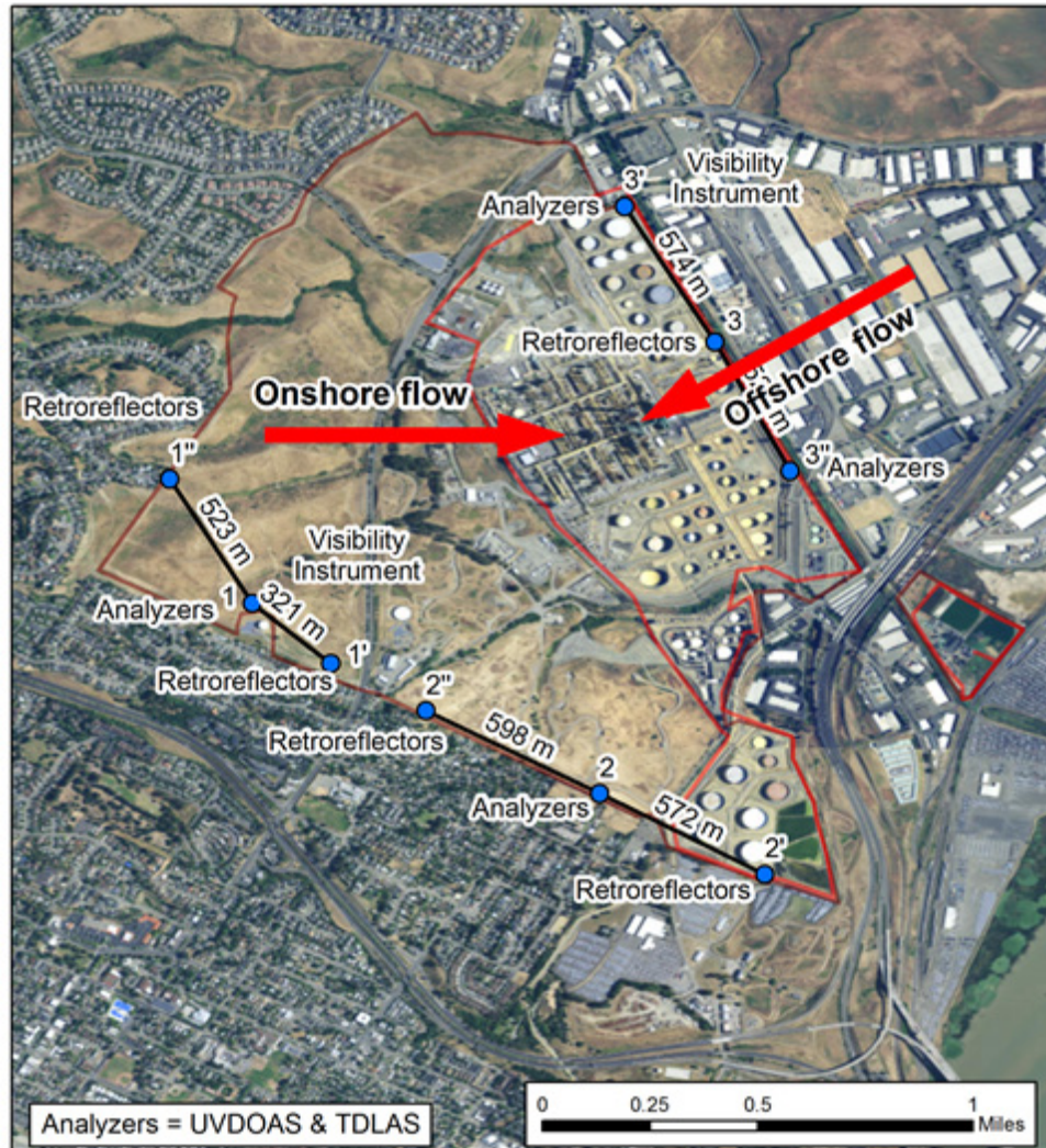
Figure 2. Proposed open-path monitoring network for Valero's Benicia Refinery. Each primary path is numbered and contains segments that are labeled with the path number and a prime (') or double prime (") symbol. Main wind flow directions are shown.
