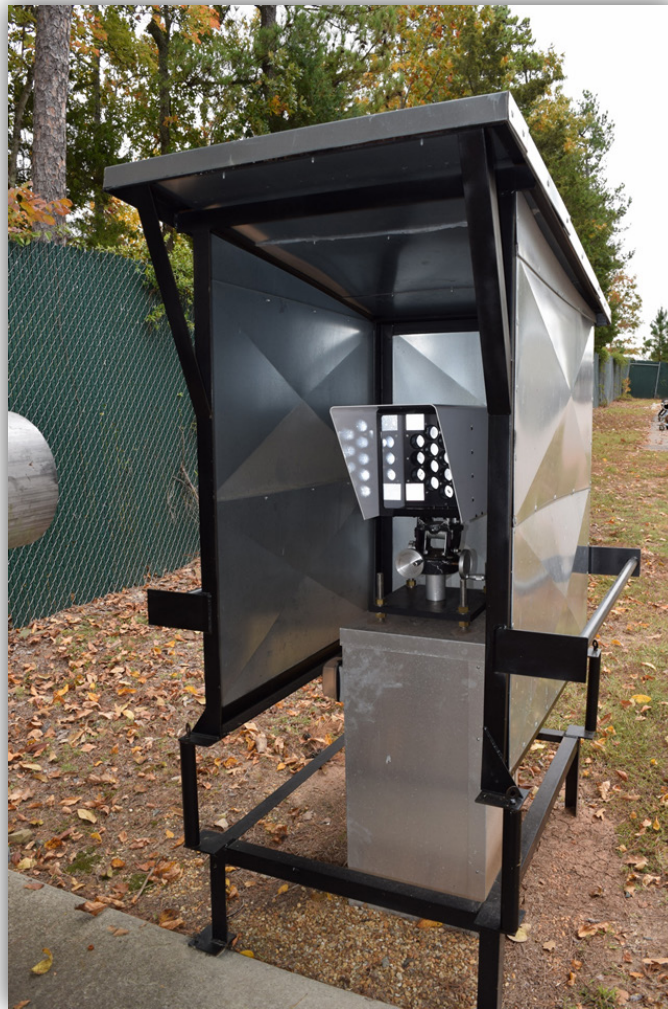
Figure 18. Example of a UV-DOAS retroreflector installation.
