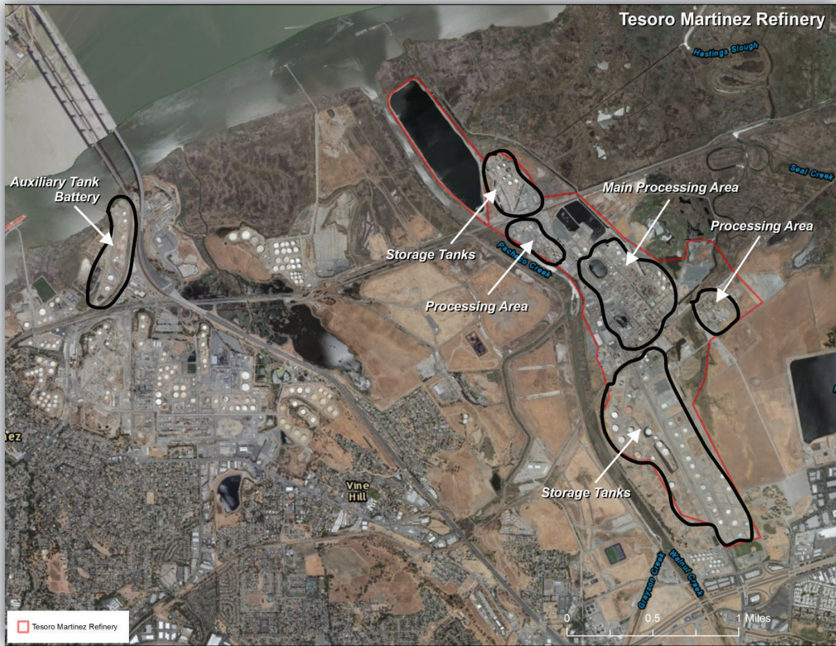
Figure 4. Layout of the Tesoro Martinez Refinery.
