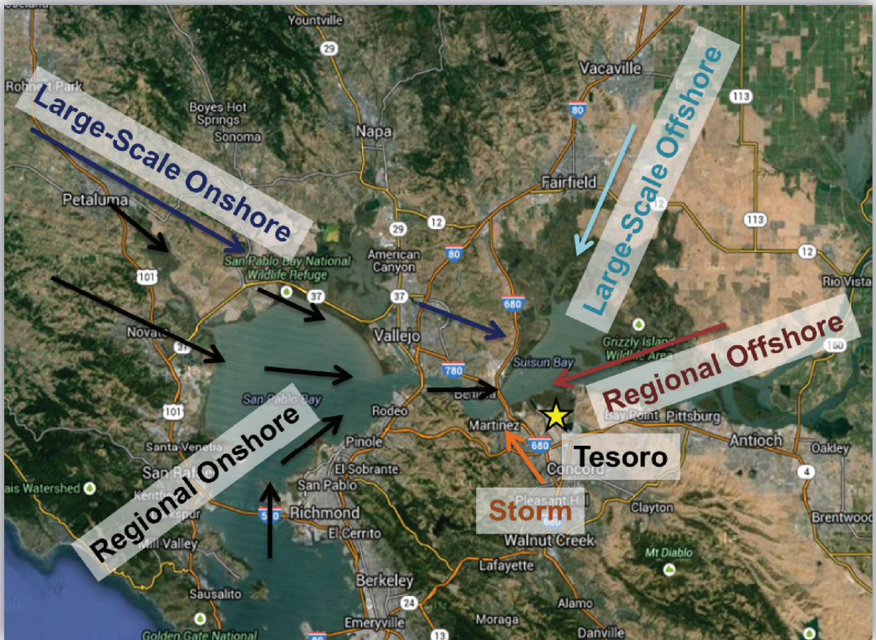
Figure 5. Typical wind flows influencing the Tesoro Martinez Refinery.
