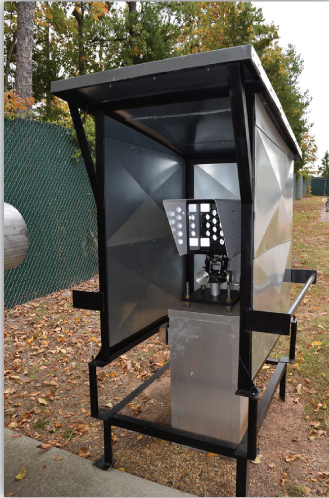
Figure 13. A UV-DOAS retroreflector.
