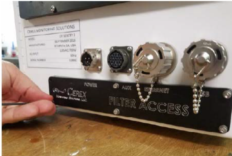
Figure A-5. Location of filter access plate.
