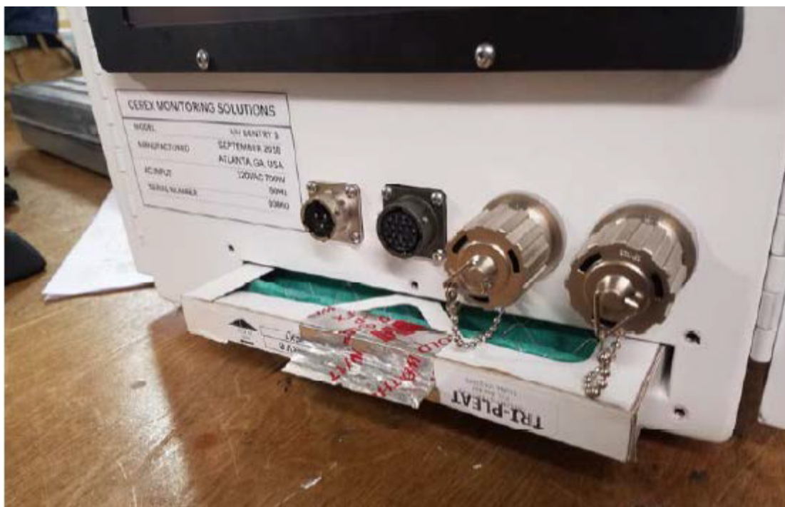
Figure A-6. Filter access plate removed and filter partially removed.
