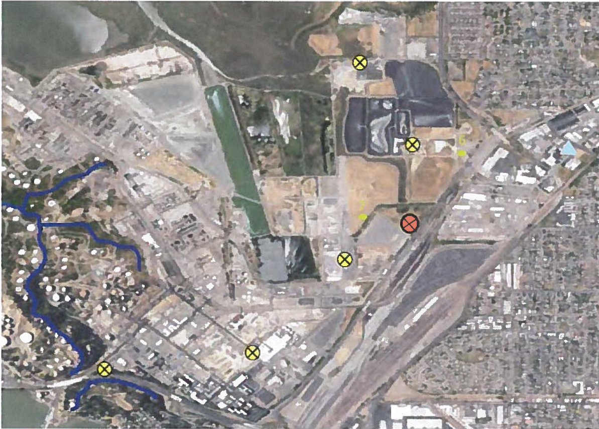
Figure 3.5 Proposed Locations of Rule 12-15 Monitors with Point FTIR Monitor Option
