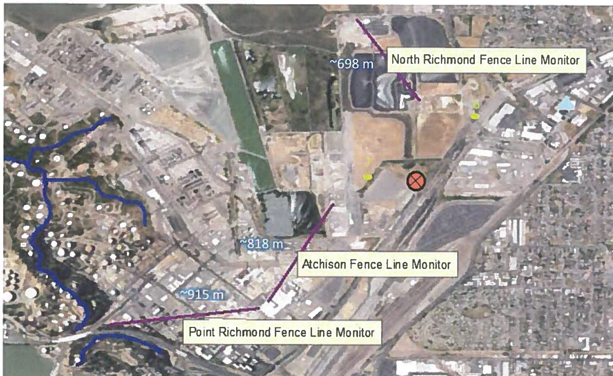
Figure 3.4 Proposed Locations of Rule 12-15 Monitors With Open Path FTIR Option
