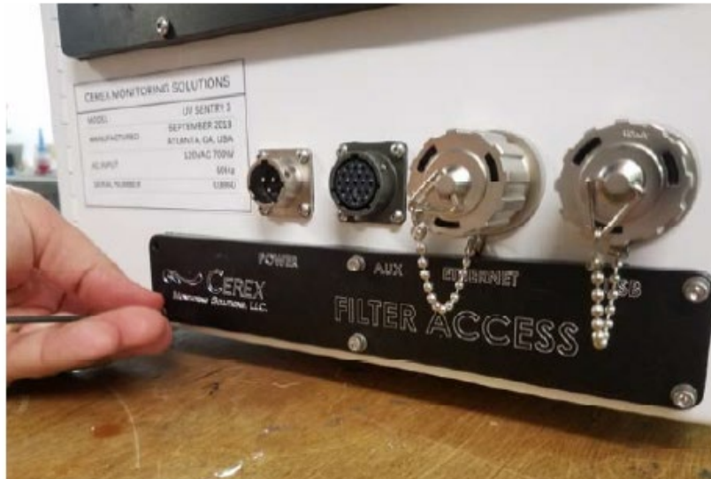
Figure A-5. Location of filter access plate.
