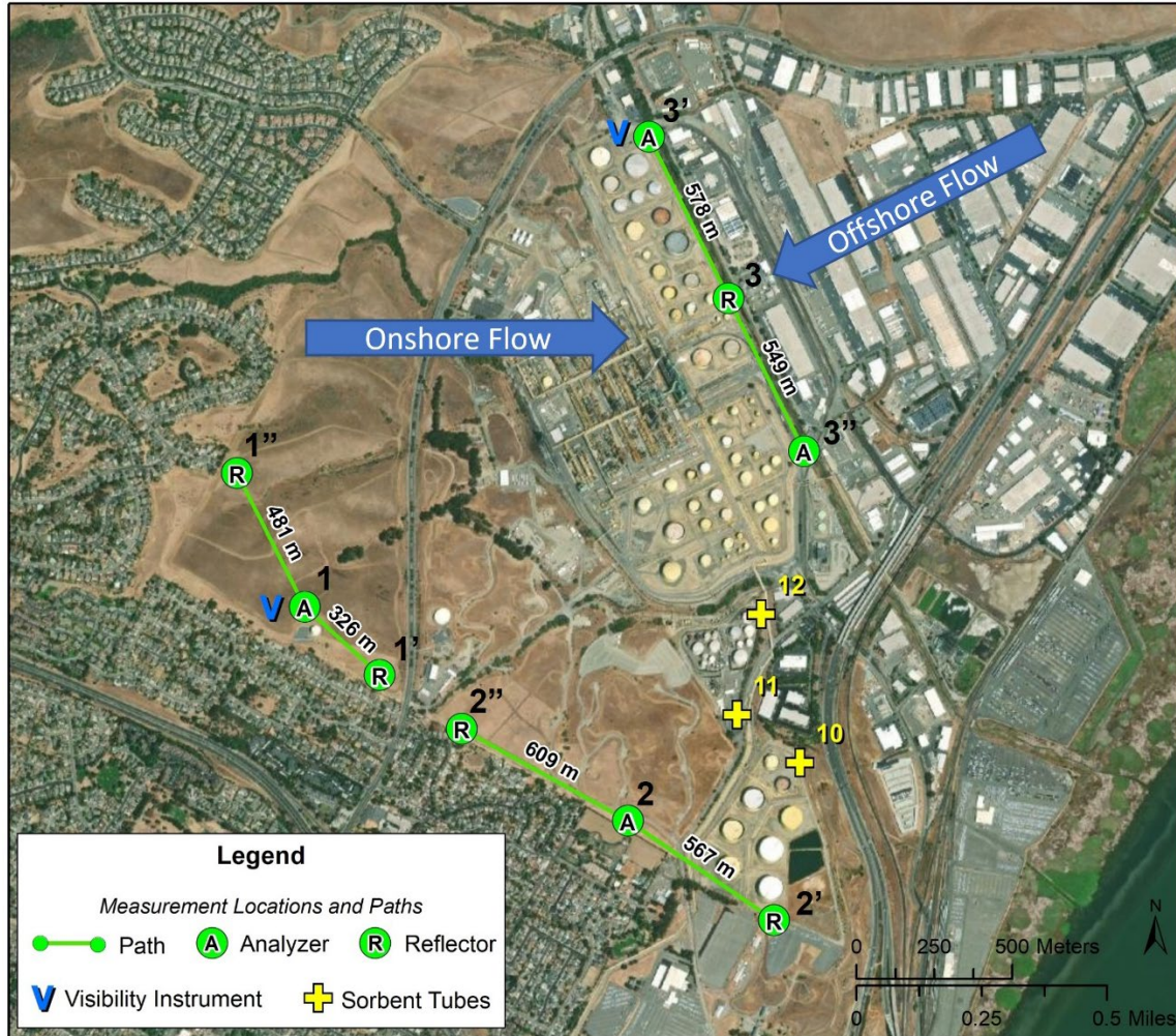
Figure 2. Open-path monitoring network for Valero’s Benicia Refinery. Each primary path is numbered, and the endpoints are numbered and labeled with a prime (') or double prime (") symbol. Main wind flow directions are shown.
