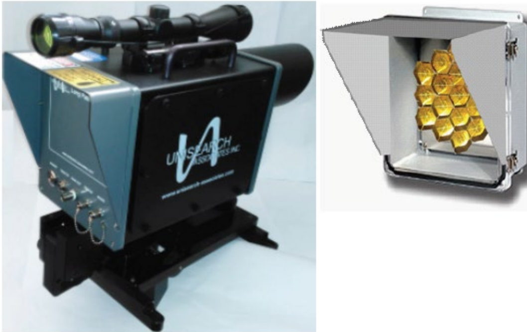
Figure B-1. Unisearch TDLAS analyzer and retroreflector array.
