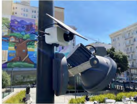
An air-quality sensor hangs in Father Alfred E. Boeddeker Park in San Francisco's Tenderloin, an effort to measure the air near impoverished communities. (Photo courtesy Brightline Defense)
