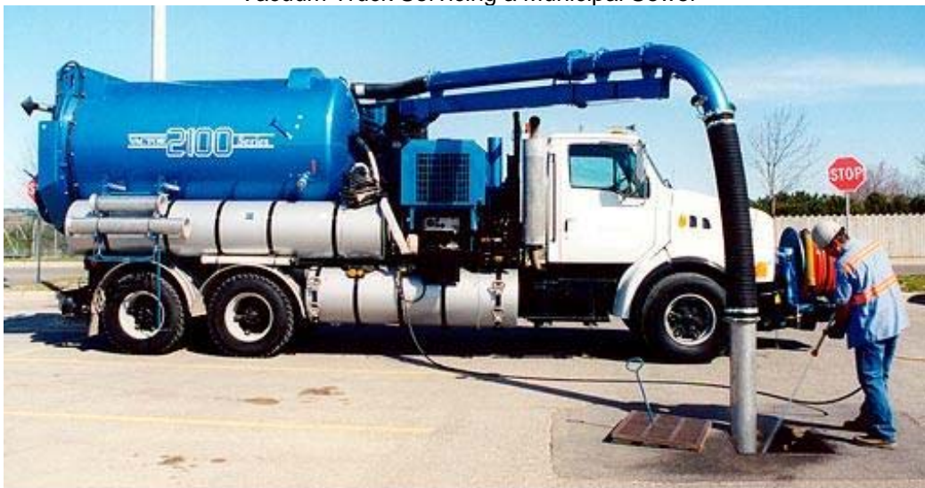
Figure 3 Vacuum Truck Servicing a Municipal Sewer
