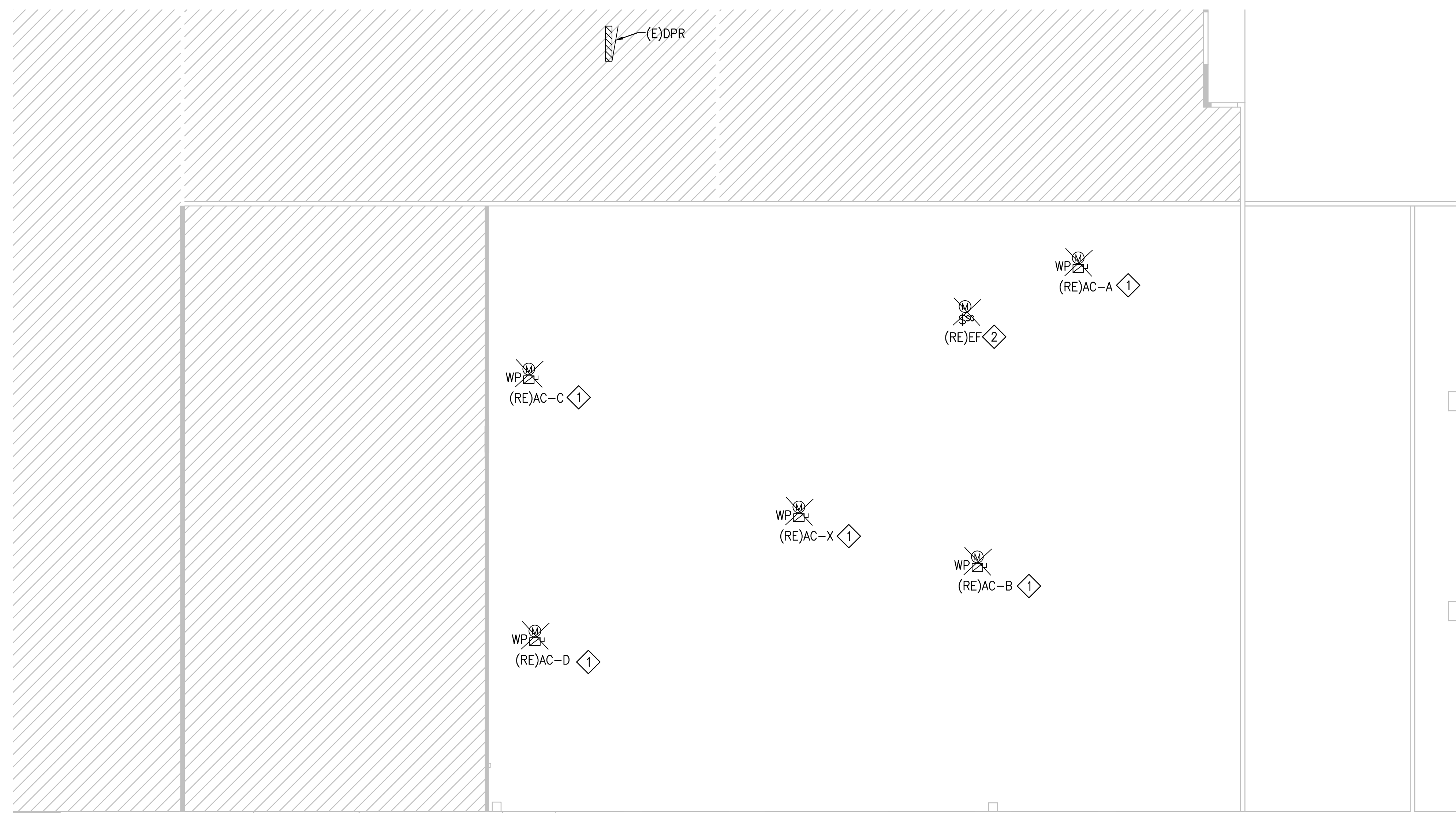
2 ROOF ELECTRICAL DEMOLITION PLAN SCALE: 1/8"=1'-0"
