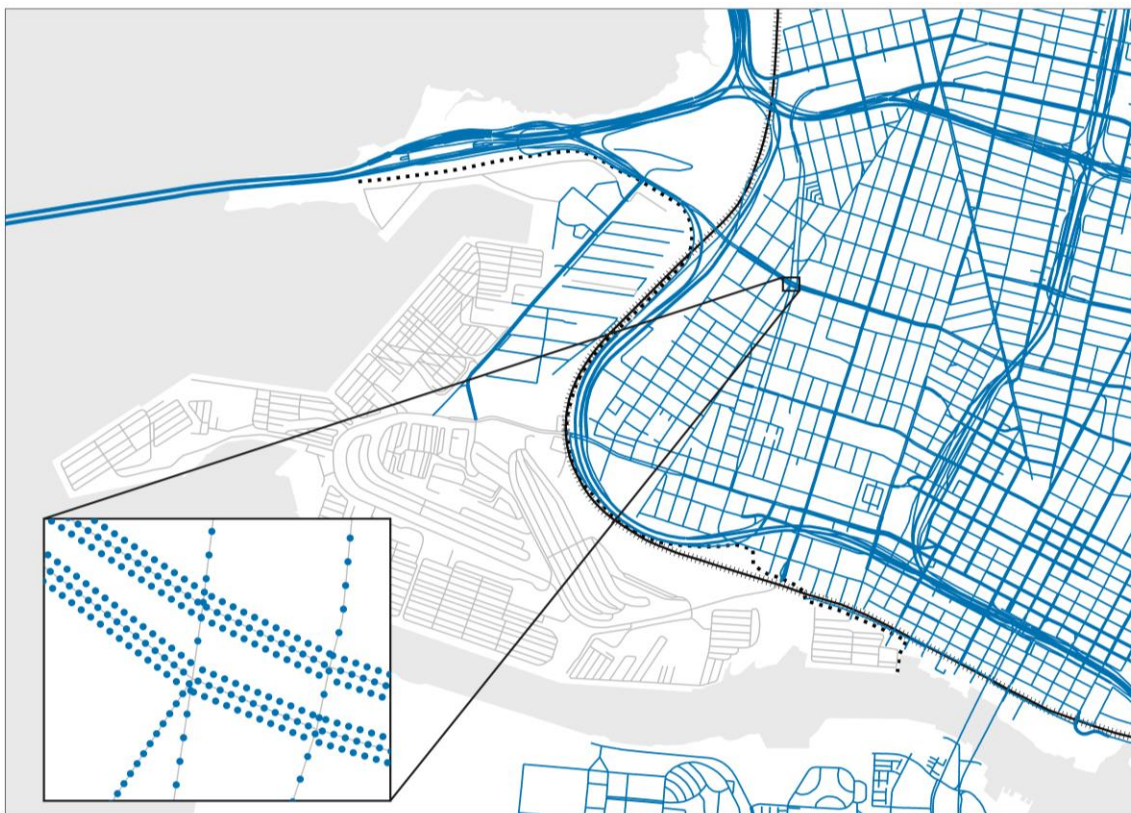
Figure 3-4. Locations of adjacent volume sources used to model emissions from on-road mobile sources. In the inset, the grey lines represent the location of roadway centerlines. The location of the marker represents the centroid of the volume source; the size of the marker does not reflect the dimensions of the volume source.
