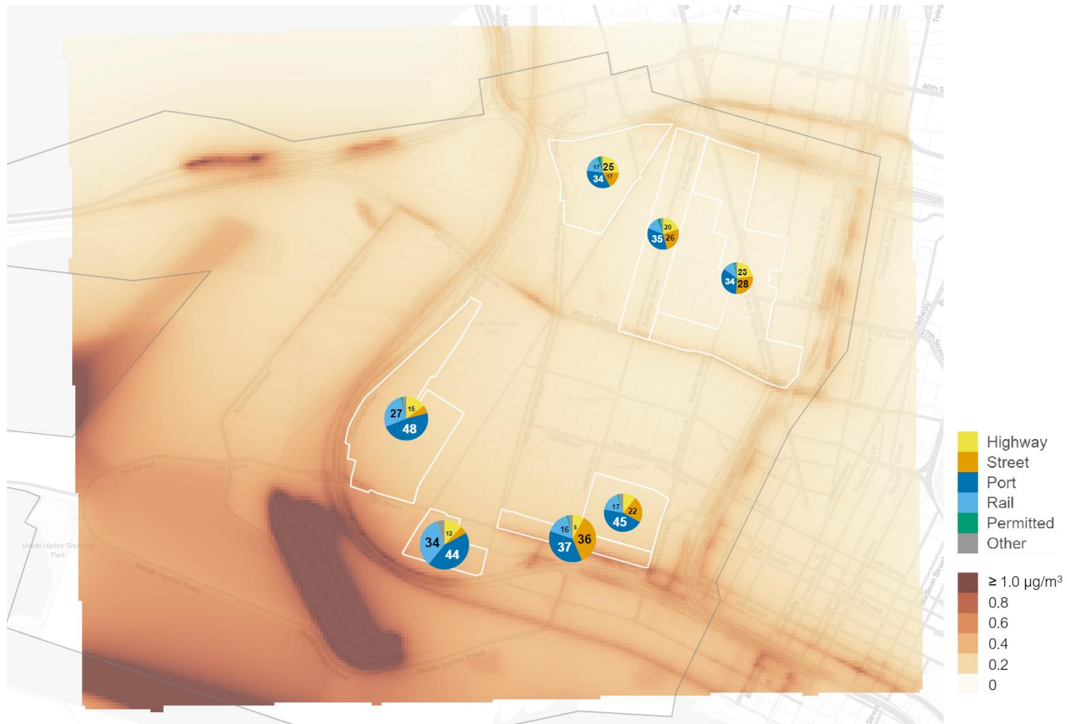
Figure 5-2. Annual average DPM concentrations associated with local sources in the West Oakland Receptor Domain (colored extents). Pie charts indicate the percentage of concentrations contributed from specific Source Categories in each zone (white polygons, Figure 4-1); the size of the pie chart indicates the total magnitude of the concentration. The grey line indicates West Oakland Community Boundary.
