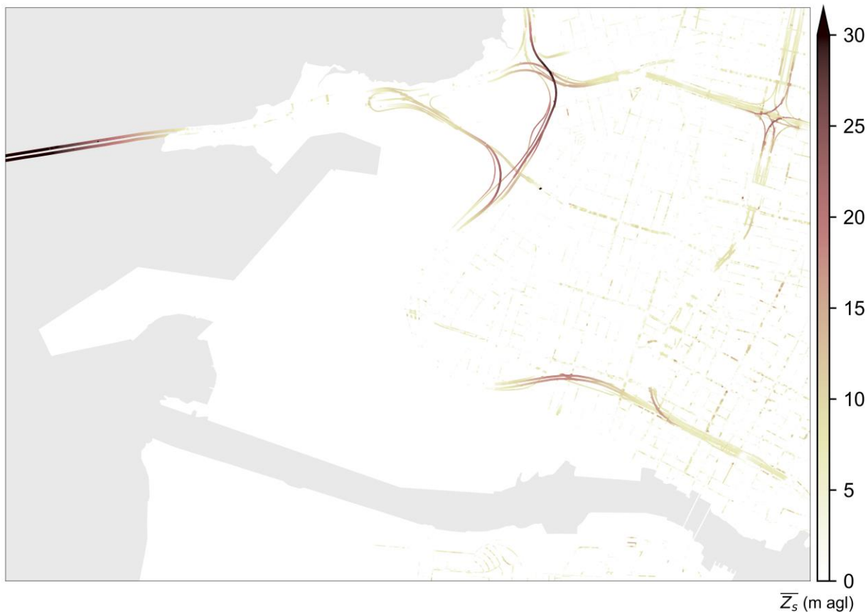
Figure 3-5. Average absolute structure heights of roadways at volume source centroids derived from lidar datasets. A \bar{Z}_s value of 0 m agl indicates (white, not visible) that the volume source is at ground level and the roadway is at grade.
