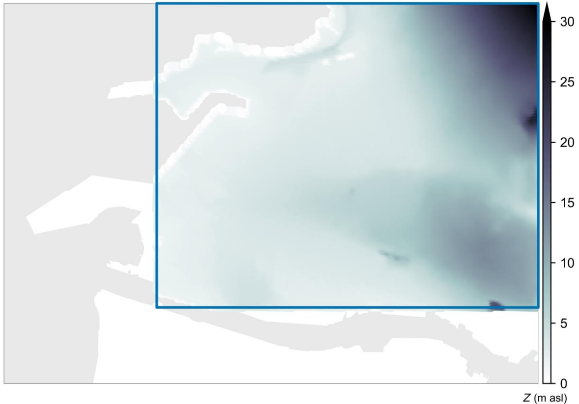
Figure 3-19. Elevation based on SRTM digital terrain data processed through AERMAP. Elevations are assigned to receptor locations only within the West Oakland Receptor Domain (blue polygon).
