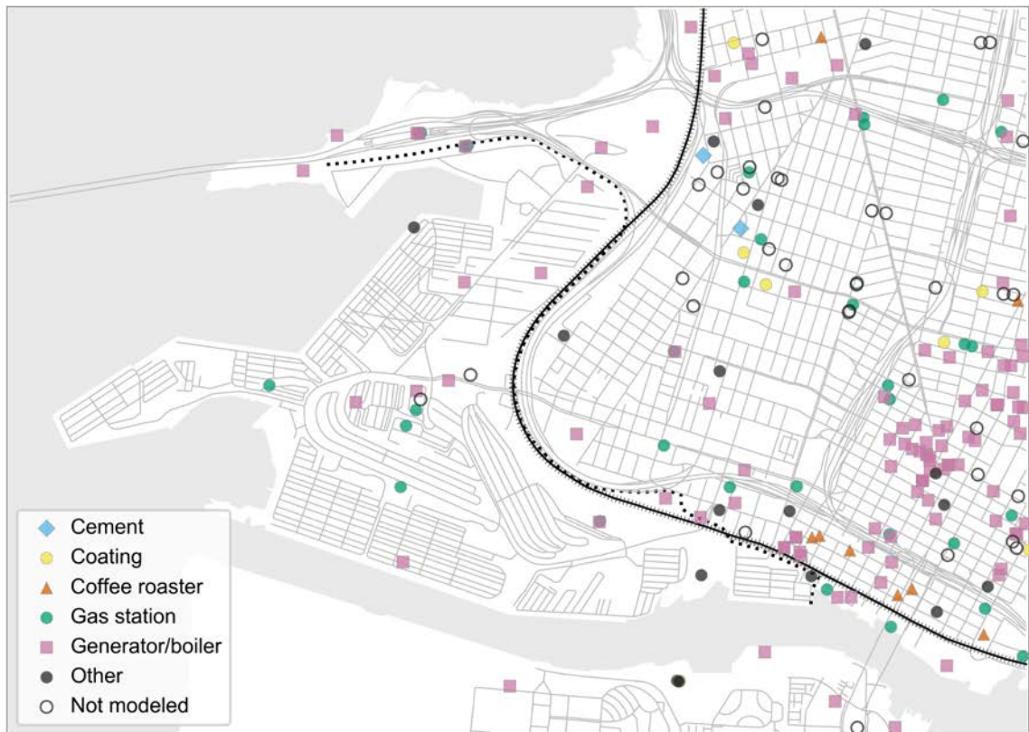
Figure 2-5. Location of permitted stationary sources in West Oakland. “Generator/boiler” indicates either a generator (primary or standby), boiler, generator and boiler, or generator and fire pump. “Other” sources include: charbroilers, cremators, electric shredders, furnaces, grain systems, microturbines, printing presses, recycling, sandblasting, smoke houses, soil vapor extraction, and turbines. Sources that were “Not modeled” were excluded because either PM_{2.5} emissions were not available, or because the TACs that are emitted do not contribute to cancer risk.
