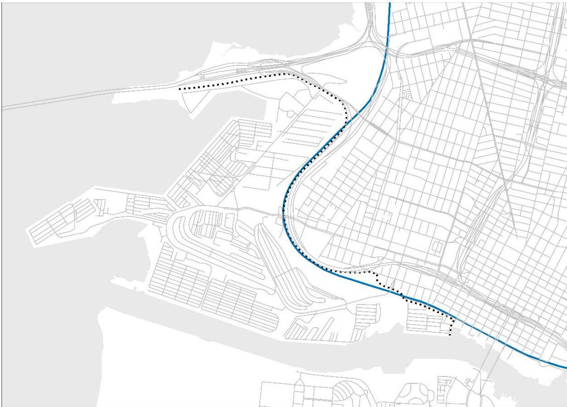
Figure 3-15. Locations of adjacent volume sources used to model emissions from locomotives. The size of the markers does not reflect the dimensions of the volume sources.
