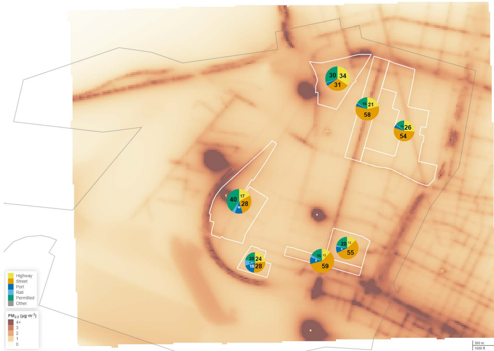
Figure 5-1. Annual average PM 2.5 concentrations associated with modeled local sources in the West Oakland Receptor Domain (colored extents) for 2024 BAU. Pie charts indicate the percentage of concentrations contributed from specific Source Categories in each zone (white polygons, Part I Figure 4-1); the size of the pie chart indicates the total magnitude of the concentration. The grey line indicates West Oakland Community Boundary. Outlines of other geographical features (roadways, etc.) are omitted.
