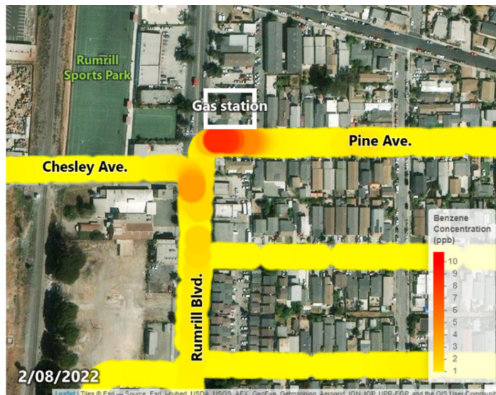
Figure 8. Relatively higher levels of benzene were measured outside the Top Gas station at Rumrill Blvd. and Pine Ave., 2/8/2022. Relatively higher levels of other VOCs were also measured at this location.
