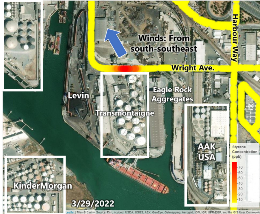
Figure 6. Relatively higher levels of styrene were measured along Wright Ave. near and downwind of the Transmontaigne tank terminal, 3/29/2022.
