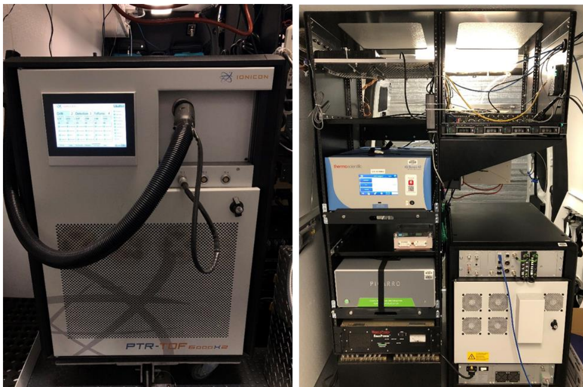
(Left) Proton Transfer Reaction Mass Spectrometer (PTR-MS), one instrument in the Air Toxics Monitoring Van that can accurately identify many different VOCs at the same time and at very low concentrations. (Right) Air Toxics Monitoring Van secondary instrumentation and data components.
