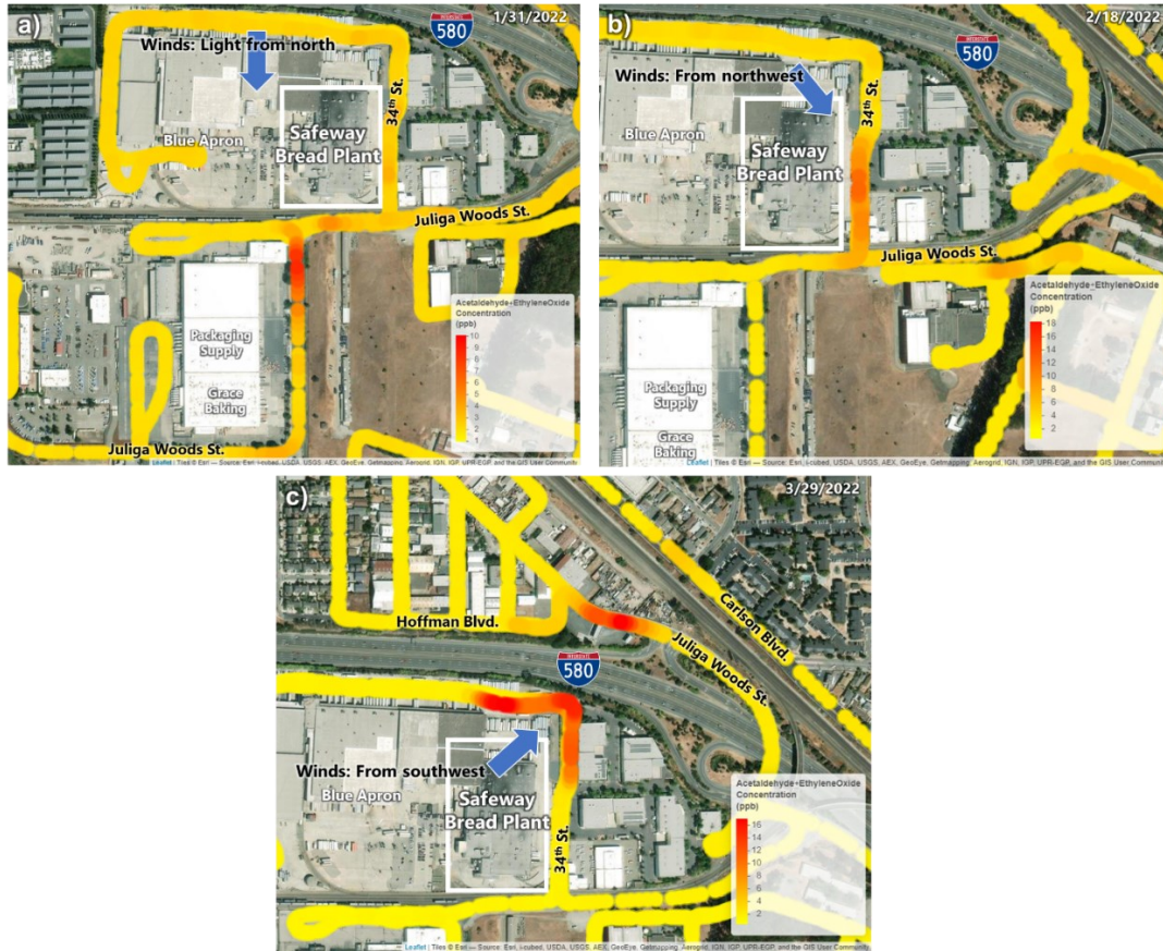
Figure 12. Relatively higher levels of acetaldehyde were measured near and downwind of the Safeway Bread Plant, as shown in a) 1/31/2022, b) 2/18/2022, and c) 3/29/2022.
