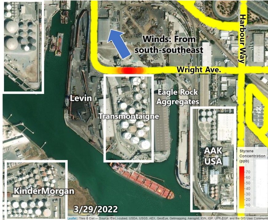
Figure 6. Relatively higher levels of styrene were measured along Wright Ave. near and downwind of the Transmontaigne tank terminal, 3/29/2022.
