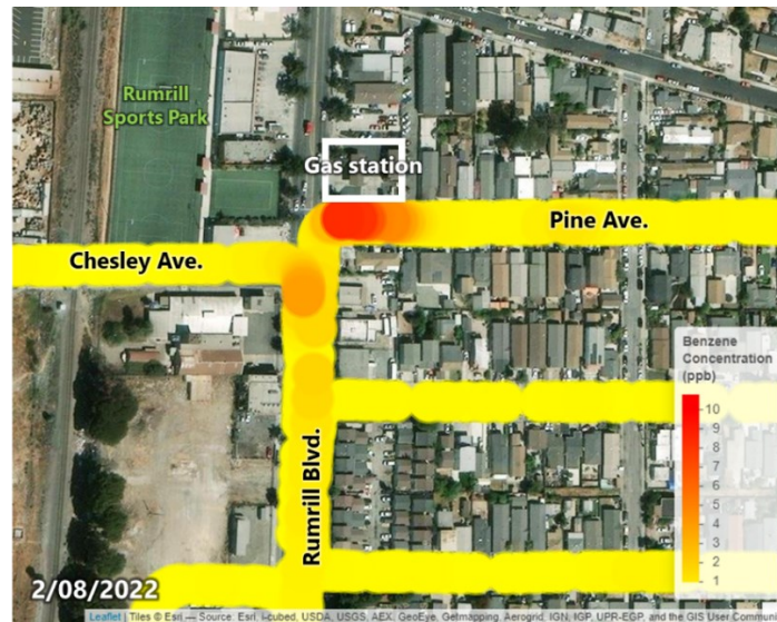
Figure 8. Relatively higher levels of benzene were measured outside the Top Gas station at Rumrill Blvd. and Pine Ave., 2/8/2022. Relatively higher levels of other VOCs were also measured at this location.
