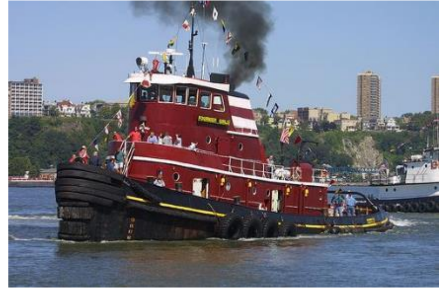
Tugboats operating offshore may have older engines and be a significant source of Diesel PM
