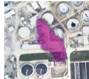
Methane plume from a sewage treatment plant
