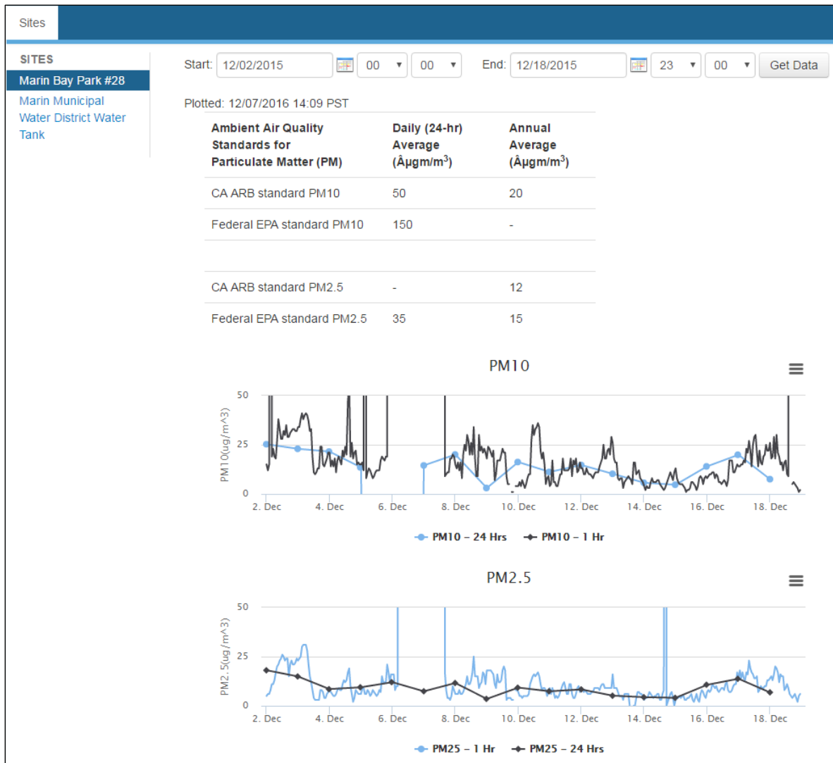
Figure 13. Example of non-public field operations website used for daily review of instrument operations.
