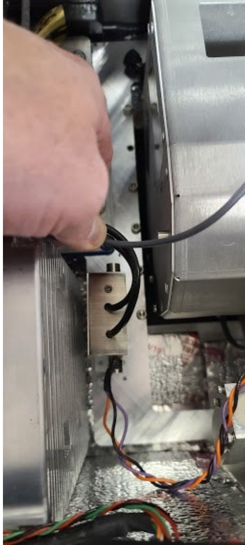
Figure 7. Preamp assembly (with orange, black and purple wires) between the heatsink (left) and interferometer (right).
